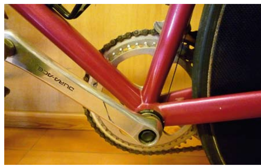
The Columbus Max tubes flatten as they approach the bottom bracket, ending in a smooth and attractive join at the shell. Anderson used 175mm Dura-Ace 7400 cranks, fitted to the square-taper bottom bracket of the day. From this angle the close-ratio chainrings are also visible.
