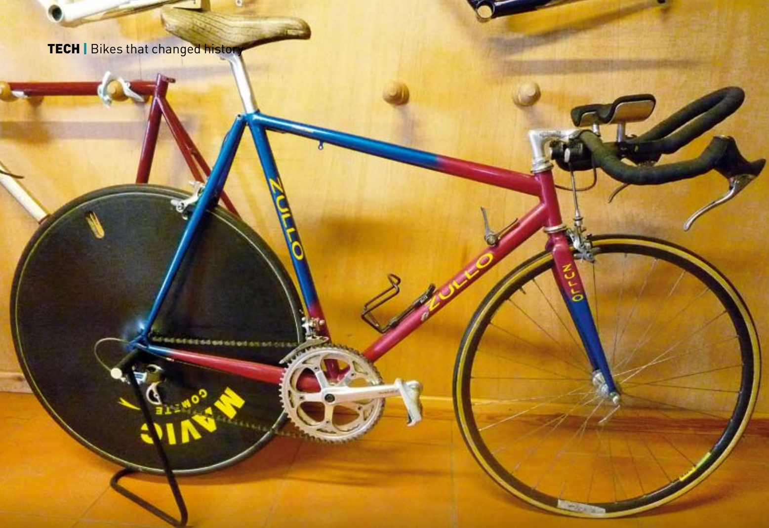
The bladed Columbus 650c fork is as aerodynamic and lightweight as it was possible to get using steel. The rest of the front end comprises a Mavic 88 24-hole radially spoked wheel with Vittoria Juniores tub and Dura-Ace caliper.
